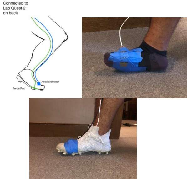
Figure 4: Experimental setup showing use of an Interlink Electronics FSR 406 (IL-406), measuring raw potential (0-5V), and a Vernier 3-Axis Accelerometer (3D) on the toe measuring downward and forward acceleration of the foot in m/s^2 . The physical setup is also shown, with the force pad taped to the runner's sock and the accelerometer taped to the top of the cleat. Both cables were taped to the runner's leg and connected to a LabQuest2 in a backpack.
